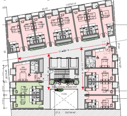
Image: Corridor length more than 40m on levels 1-9.
